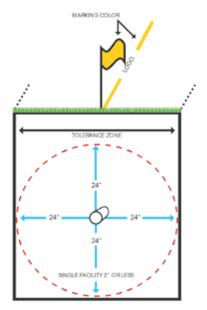
OAR 952-001-0010 (25) "Tolerance Zone" means the area within 24 inches surrounding the outside dimensions of all sides of an underground facility.
